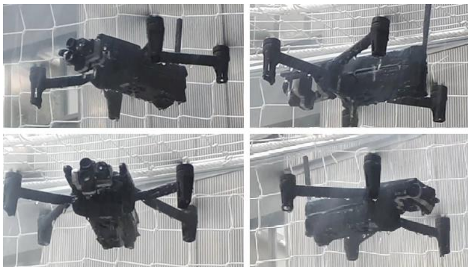
Fig. 6: IPX3 test (spraying 10 liters by minute)
