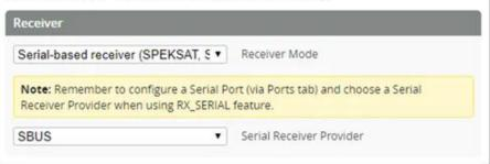
Note: The HD digital VTX has an integrated SBUS receiver which works with the DJI radio. If you are using an external receiver, then you do not need to wire SBUS to the digital VTX. Instead, connect the external receiver as indicated above.
